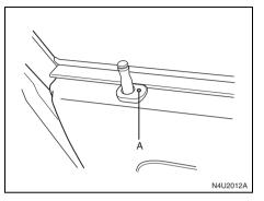
The security light (A) will flash once every 0.8 seconds to indicate that the theft-deterrent system is armed. The security light is located on the driver's door lock.
